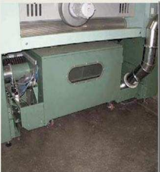
Waste disposal box for discontinuous suction of waste from the licker-in
